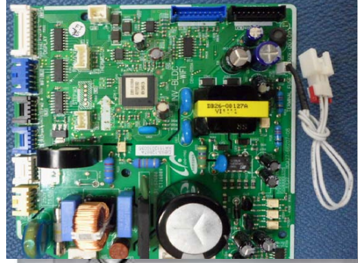
Connection of terminal block and Main PBA
